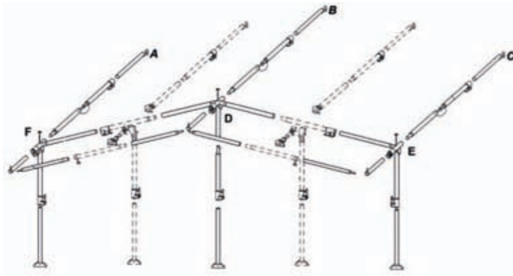
Pole assembly diagram of an awning with canopy roof (incl. pole reinforcement)
